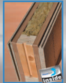
Model - Timber Stud Wall. PhoneStar screwed to the studs and plasterboard screwed to the PhoneStar
